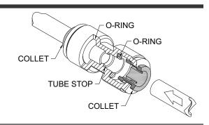
Pull on the fitted Tubing to ensure it is secure.
