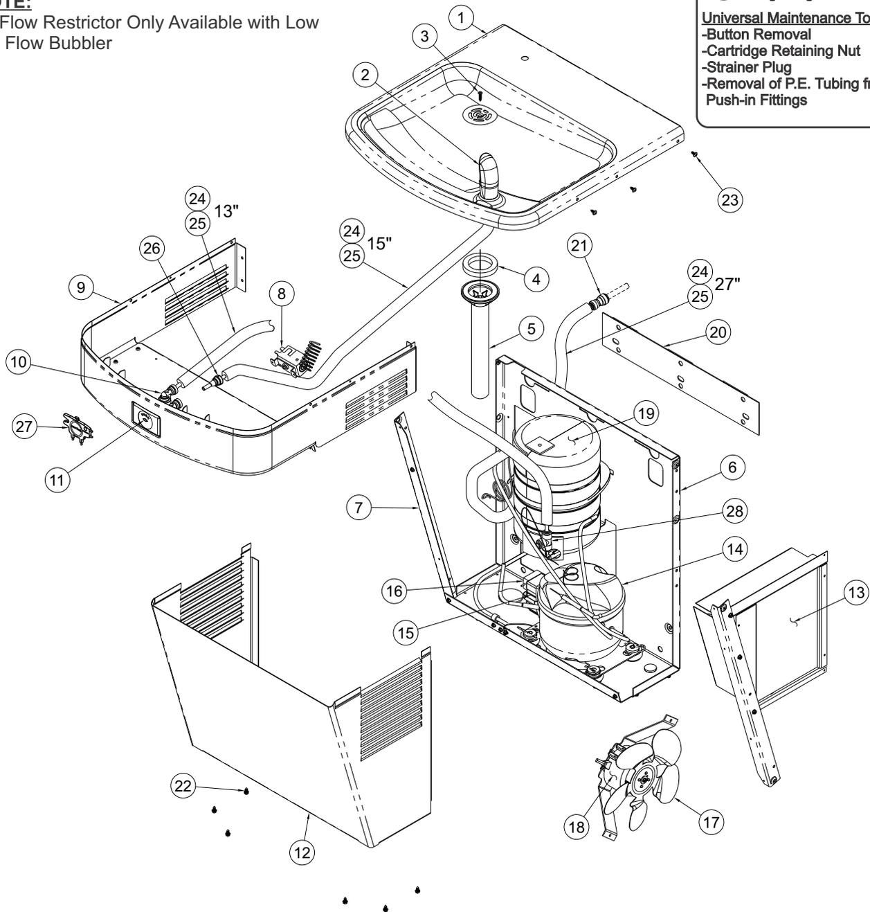
Standard A171.8-UG-BF<sub>x</sub>S series refrigerated ADA Water Cooler shown. All 1/4" O.D. Plastic Tubing (24) must be insulated with (25) foam insulation.
