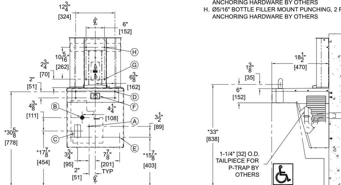
**NOTES:** Dimensions indicated (\*) are for ADA frontal approach installation. Adjust vertical dimension (\*) as required to comply with federal, state, and local codes. For Child ADA compliant parallel approach, decrease Bubbler spout height to 30" maximum above finished floor. Provide clear floor space as required.
